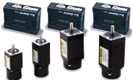
Compact and miniaturized closed loop stepping motor and drive system which utilizes a high resolution encoder to update the motor position every 25 micro-seconds. Optimizing high performance DSP technology(Digital Signal Processor) and proprietary software, the drive ensures exact position, no overshooting and smooth motion at 100% of load.
