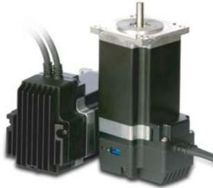
High speed, high precision drive and stepping motor integrated into one package, Ezi-STEP<sup>®</sup> is unique as it adopts a new control scheme based on a built in high performance DSP(Digital Signal Processor) and software. Ezi-STEP<sup>®</sup> utilizes a unique position estimation algorithm which instantaneously detects out of synchronization of the stepping motor rotor, which is not available with conventional stepping motor & drives.
